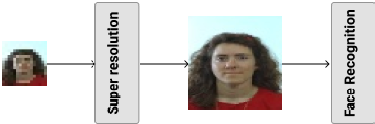
Figure 2.2: A two step workflow for face recognition which involves super resolution of the input LR image.
