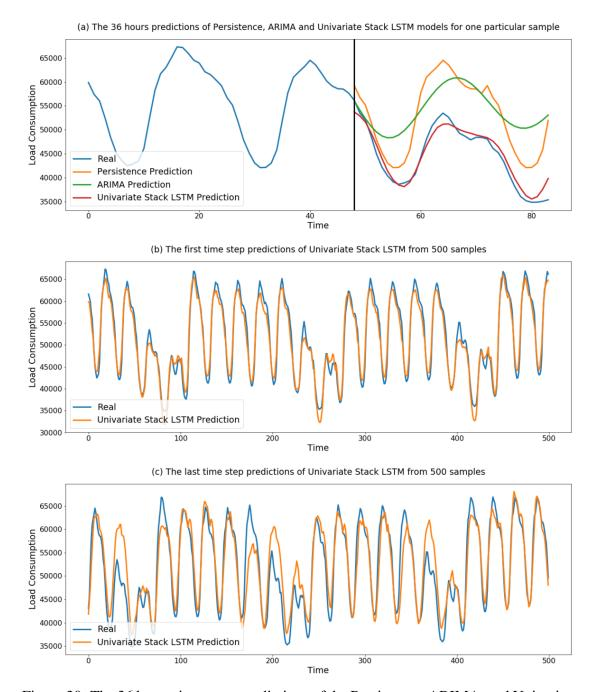
Figure 30. The 36 hours time steps predictions of the Persistence, ARIMA, and Univariate Stack LSTM models for one particular sample (a), the first time step predictions (b) and the last time step predictions (c) of the Univariate Stack LSTM model from 500 samples of Open System Load Consumption.
