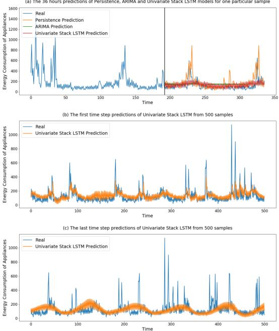
(a) The 36 hours predictions of Persistence, ARIMA and Univariate Stack LSTM models for one particular sample
