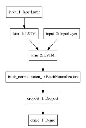
Figure 23. Encoder Decoder LSTM model.
