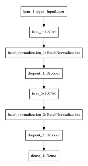
Figure 24. Stack LSTM model.
