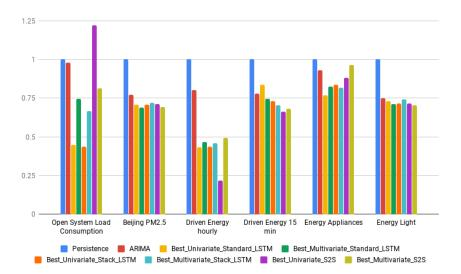
Figure 27. In the result of parameter tuning, the average scaled RMSE error relative to Persistence.
