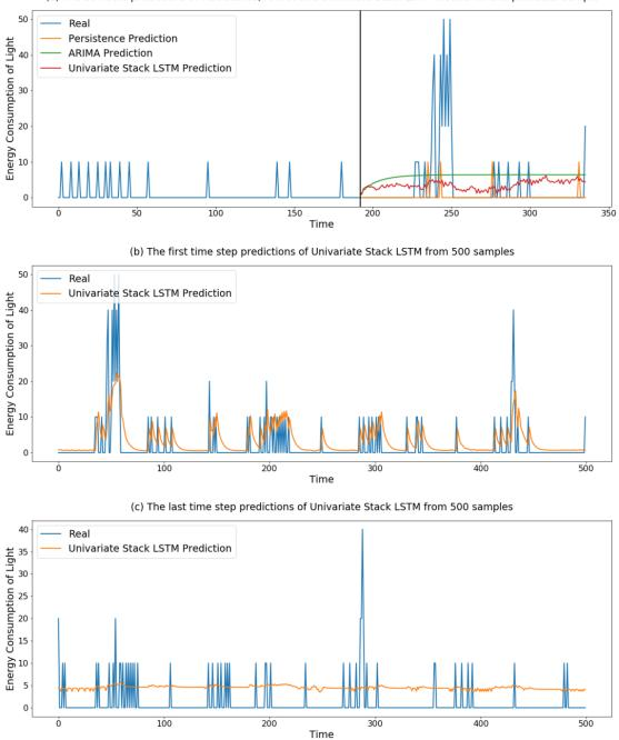
(a) The 36 hours predictions of Persistence, ARIMA and Univariate Stack LSTM models for one particular sample
