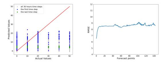
(a) The scatter plot of the actual values and pre-(b) The RMSE errors for the 36 hours forecast dictions points
