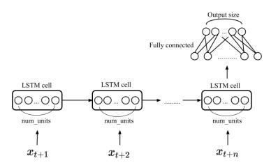
Figure 4. Standard LSTM architecture.
