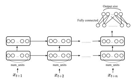
Figure 5. Stack LSTM architecture.
