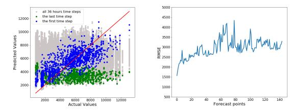
(a) The scatter plot of the actual values and pre-(b) The RMSE errors for the 36 hours forecast dictions points
