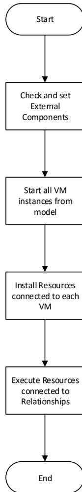
Figure 2. CloudML deployment process
