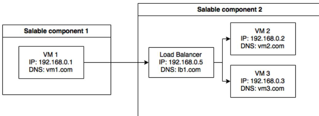
Figure 5. Representation of the deployment mode after scaling up
