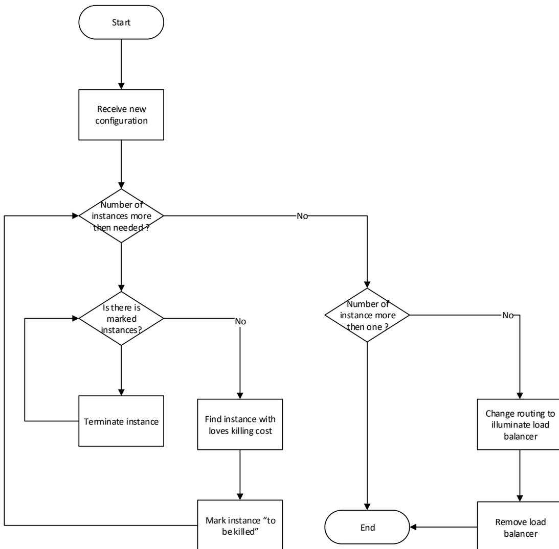
Figure 6. Scaling down algorithm
