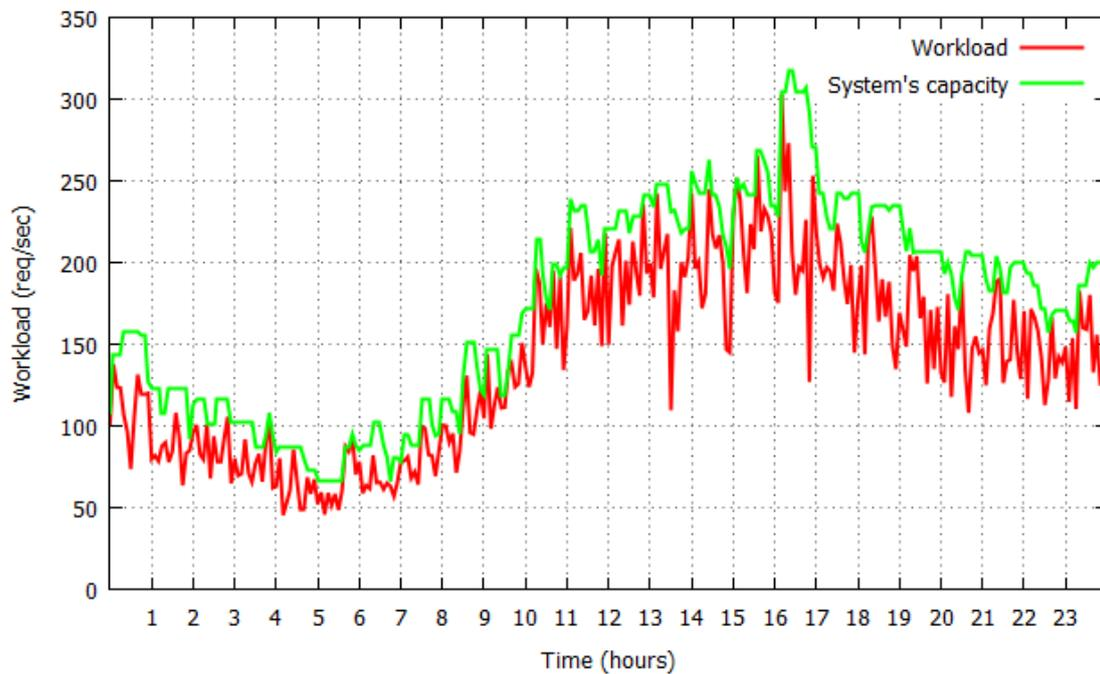
Figure 19. Workload and system capacity during parallel workflow experiment second component
