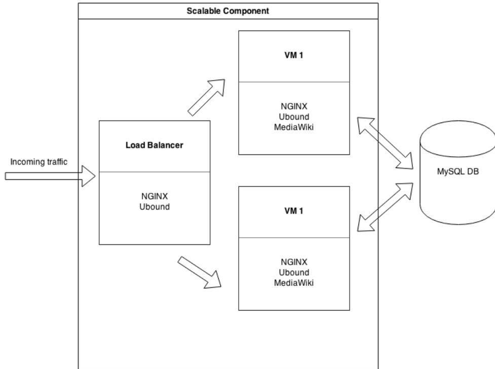
Figure 10. One component deployment configuration in case of increased workload
