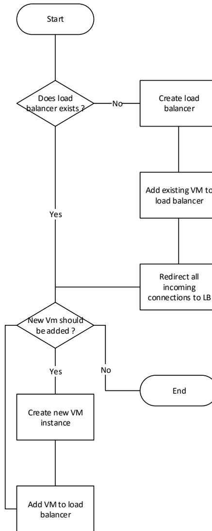
Figure 3. Scaling up algorithm
