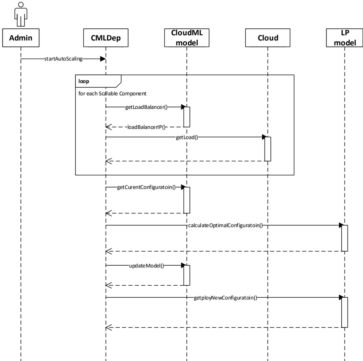
Figure 8. Auto scaling sequence diagram.
