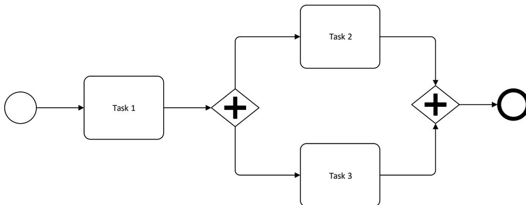
Figure 13. Example of parallel workflow
