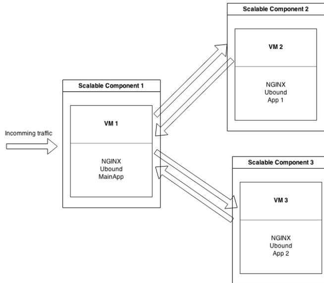
Figure 15. Initial deployment model from experiment with multiple scalable components
