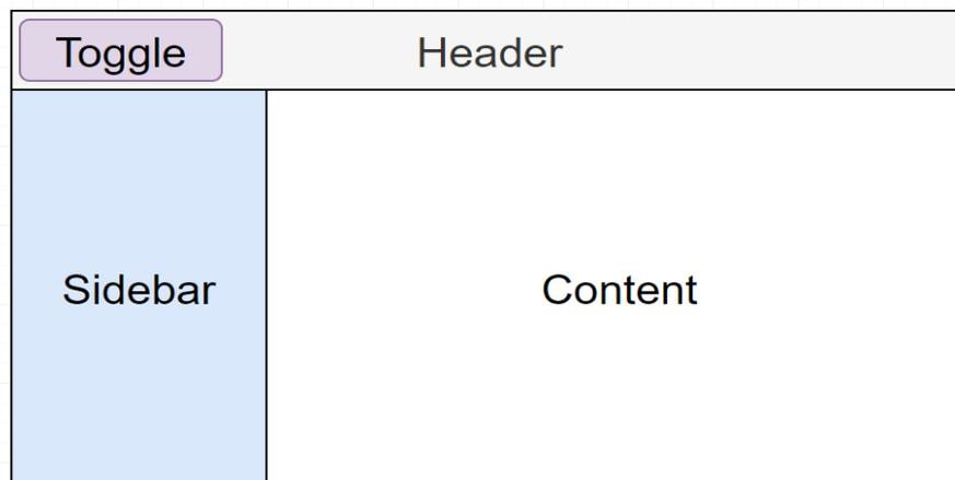
Figure 7. Layout of the Admin Tool: Header (gray), Menu (blue), Content (white) and a button to toggle the Menu (violet).
