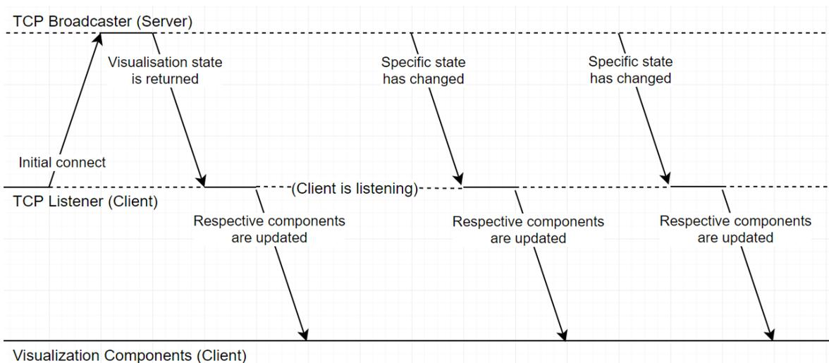
Figure 4. The communication process.
