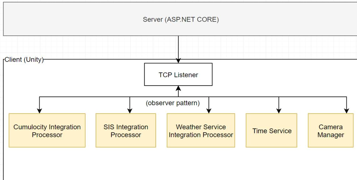
Figure 3. Components of the observer pattern: subject (white) and observers (yellow).
