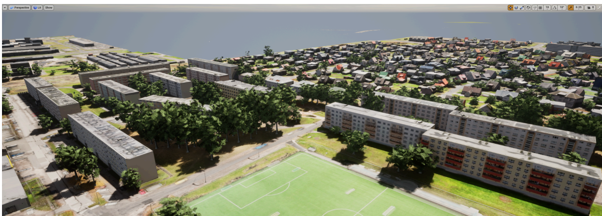
Figure20: Unreal Engine's world scene, where the implementation of Level of Detail (LOD) settings and visibility optimisations is evident through the selective rendering of objects based on their distance from the viewer. Trees, street lights and ground areas are not rendered when they are far from the camera.
