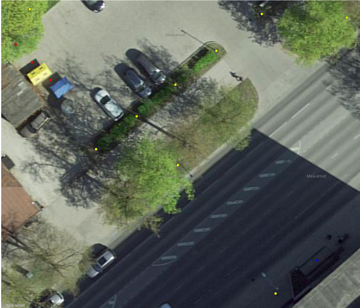
Figure 17: QGIS desktop application showing locations of imported street lights (yellow), bus stops (blue) and trash containers (red) as dots.
