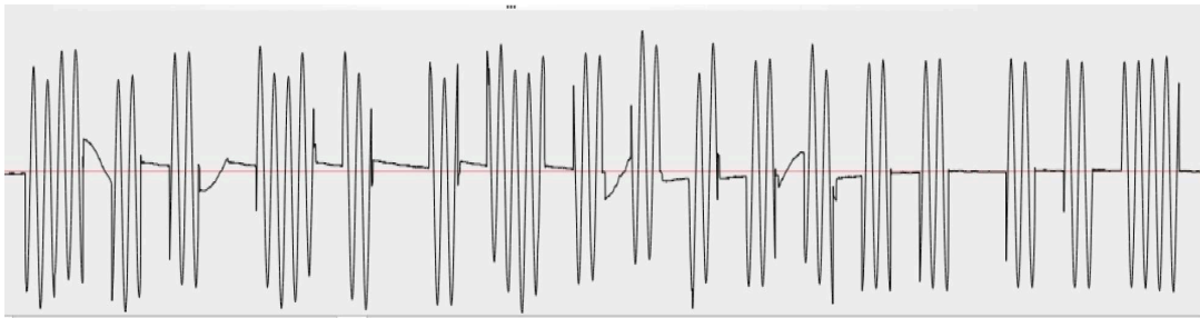
Figure 29. Jablotron keypad signal partially overlapping with weak hub signal.
