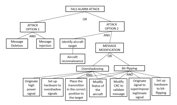
Figure 15. False Alarm Attack Tree.
