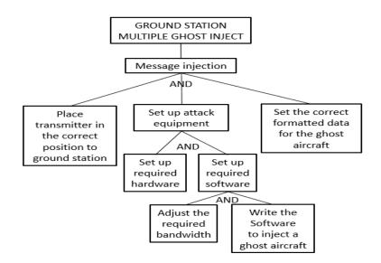
Figure 10. Ground Station Target Ghost Inject Attack Tree.
