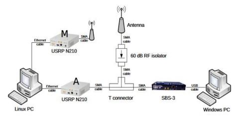
Figure 4. Experimental Hardware Set-Up to Perform Attacks Against ADS-B[57].
