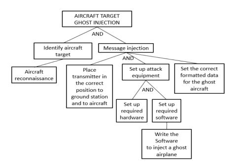
Figure 8. Aircraft Target Ghost Inject Attack Tree.
