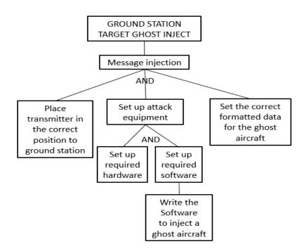
Figure 9. Ground Station Target Ghost Inject Attack Tree.
