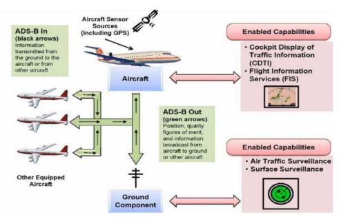
Figure 2. ADS-B Functional Diagram [51].
