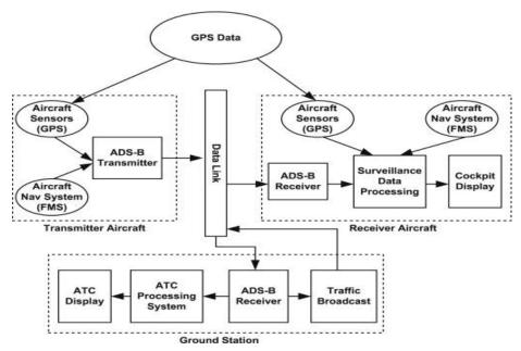
Figure 1. Main Components of ADS-B [7].
