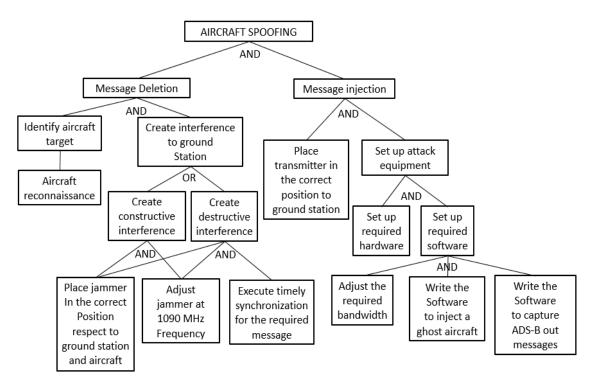
Figure 12. Aircraft Spoofing Attack Tree.
