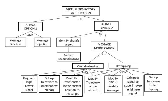
Figure 13. Virtual Trajectory Modification Attack Tree.
