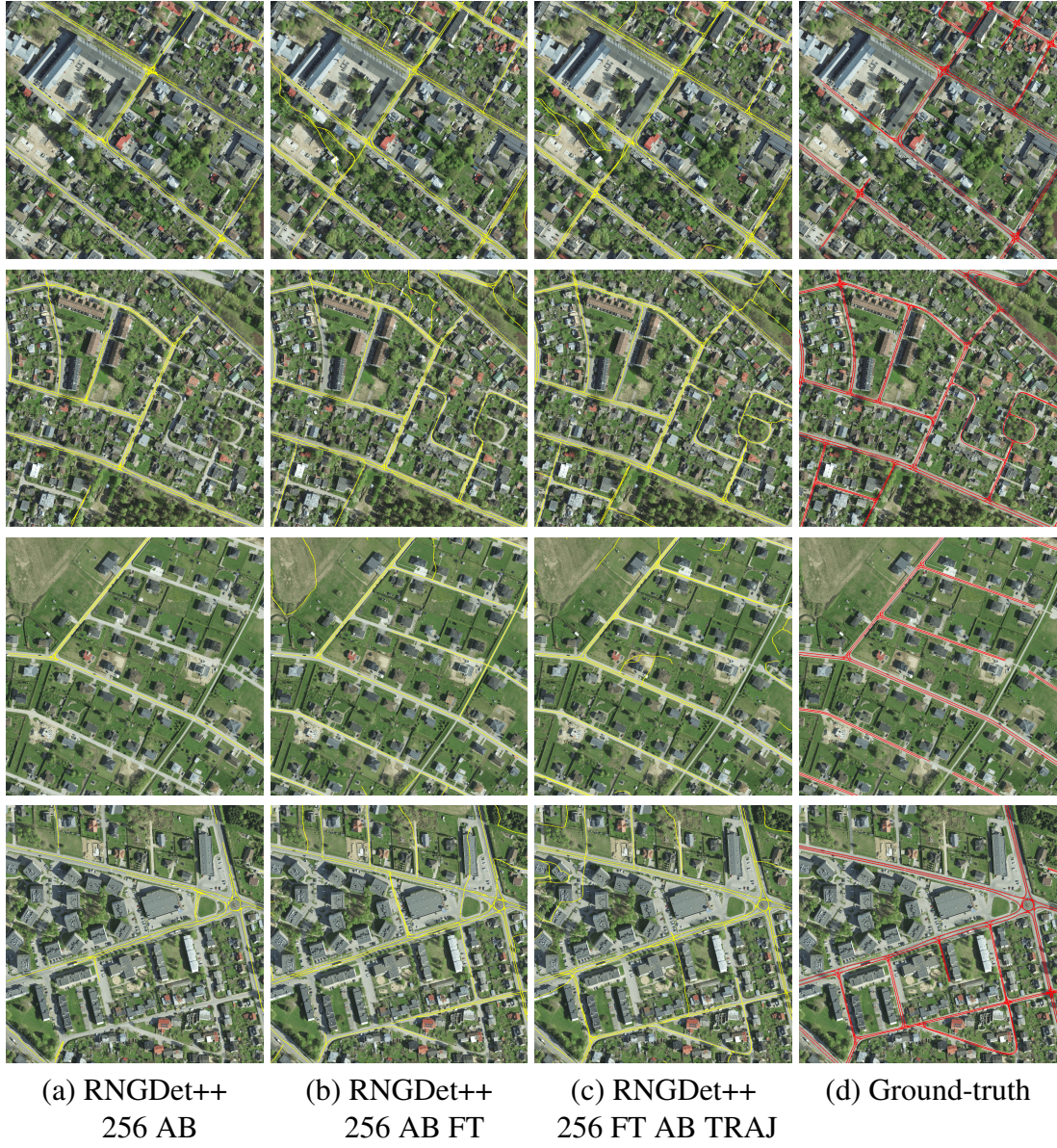
Figure 17. Sample predictions from lane detection models with \text{ROI} = 256 . Models with letters AB had an additional backbone for intersection detection. FT indicates that the models were fine-tuned on the road detection model. TRAJ denotes the model that used raw lane trajectories on input images. Orthophotos are from the Estonian Land Board. Best viewed with digital zoom.
