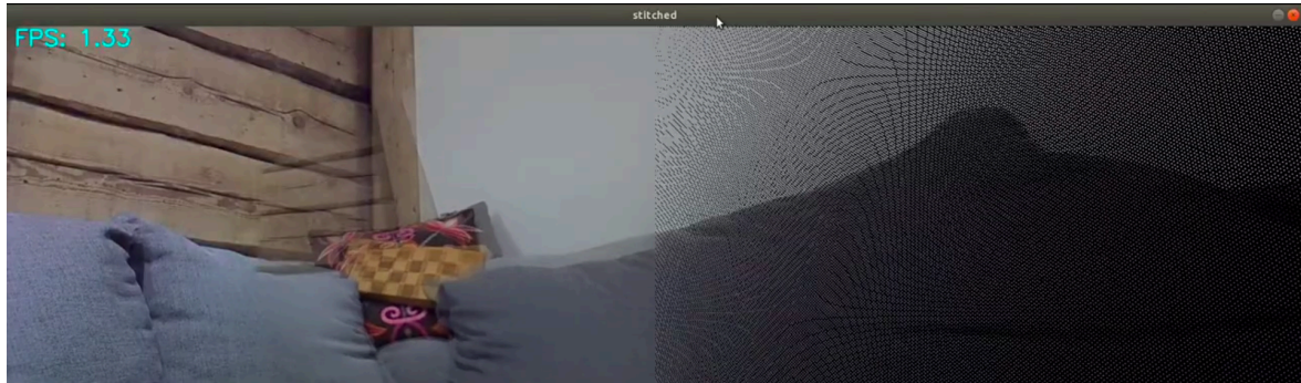
Figure 20: Stitched camera feed using SURF and OpenMP
