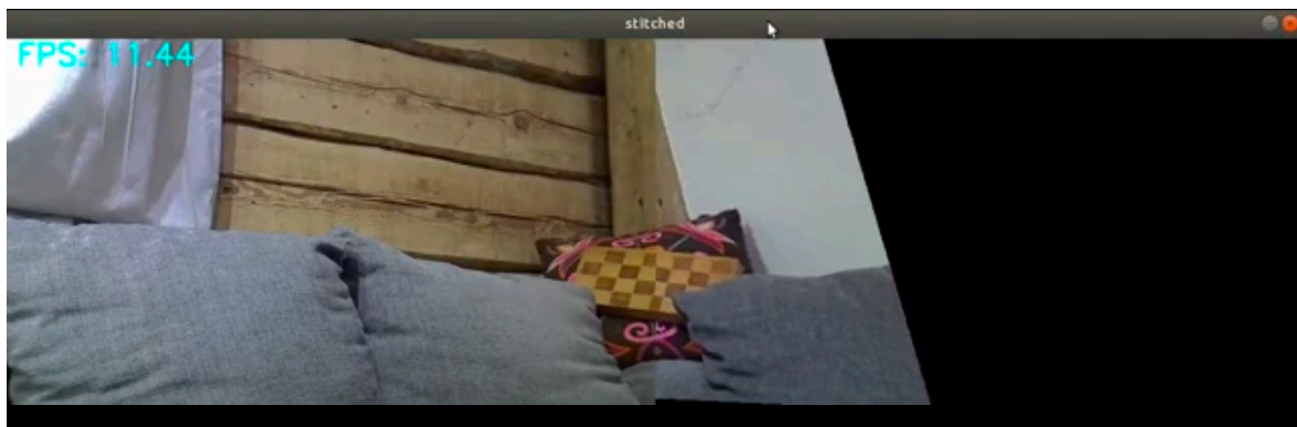
Figure 21: Stitched camera feed using SURF and OpenACC
