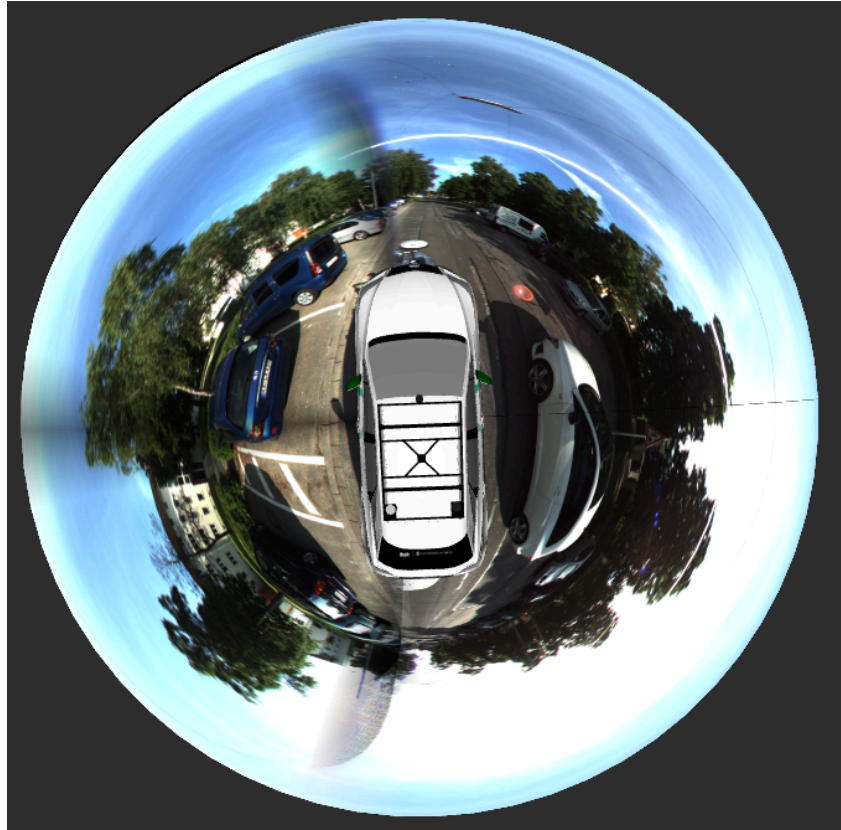
Figure 14: Dual fisheye camera images projected on a hemisphere mesh at a bird's-eye view angle.
