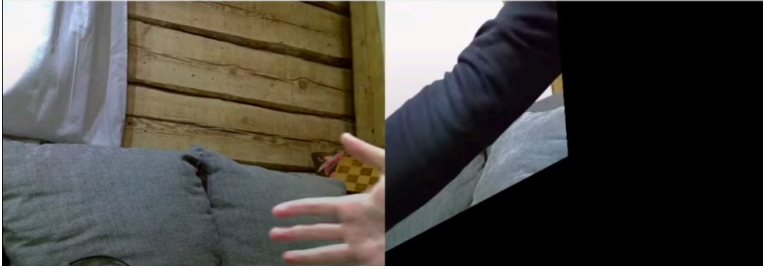
Figure 22: Unstable stitched image using SIFT and OpenACC.
