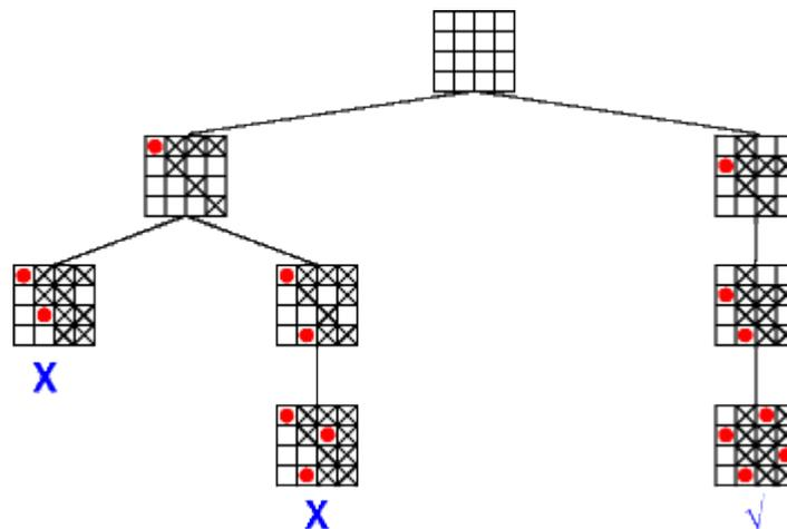
Figure 4: An example of forward checking for 4-queens problem [14]
