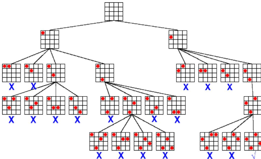
Figure 3: An example of backtracking for 4-queens problem [14]
