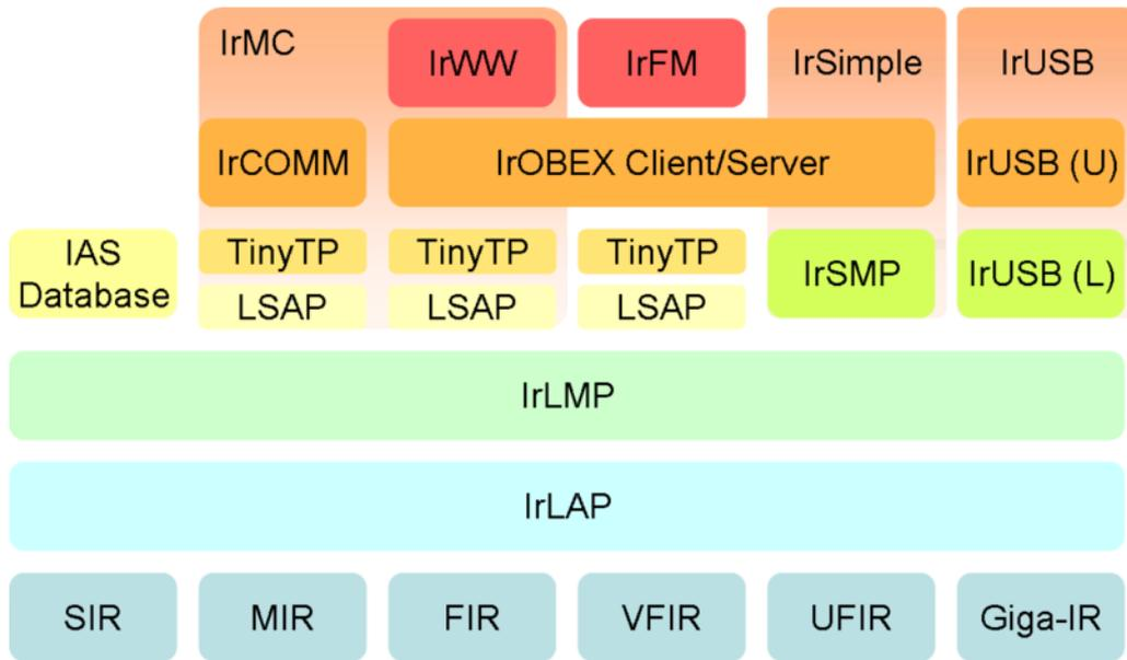
Figure 5. The IrDA protocol stack layers [20].
