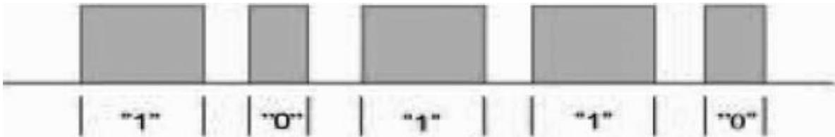
Figure 10. Pulse-length coding [23].
