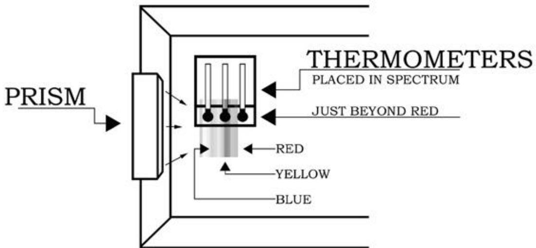
Figure 3. Thermometer setup of Herschel's experiment [7].
