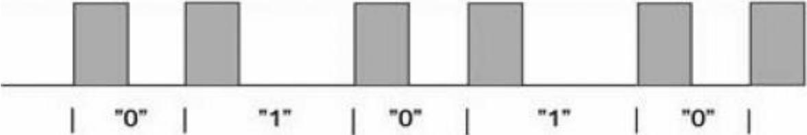
Figure 8. Pulse-distance coding [23].
