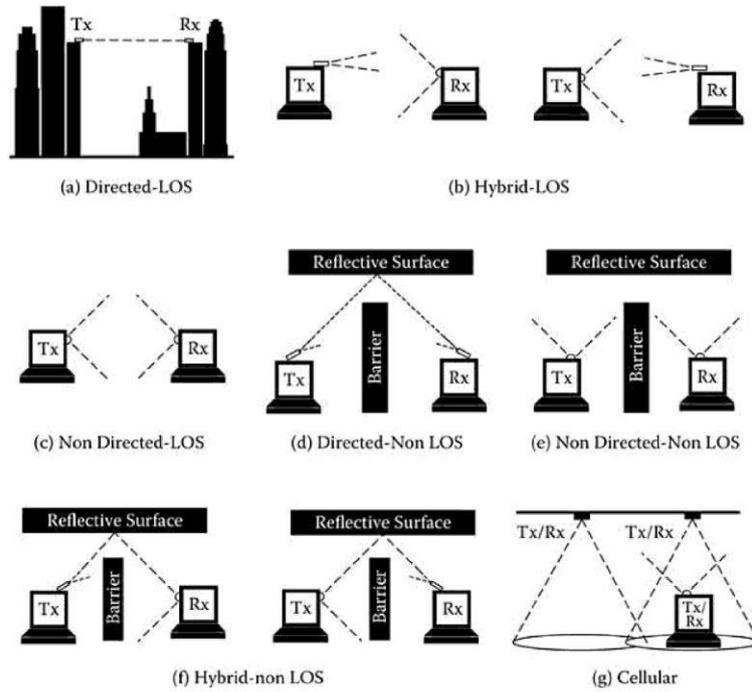
Figure 5. Different configurations of wireless IR links [19].
