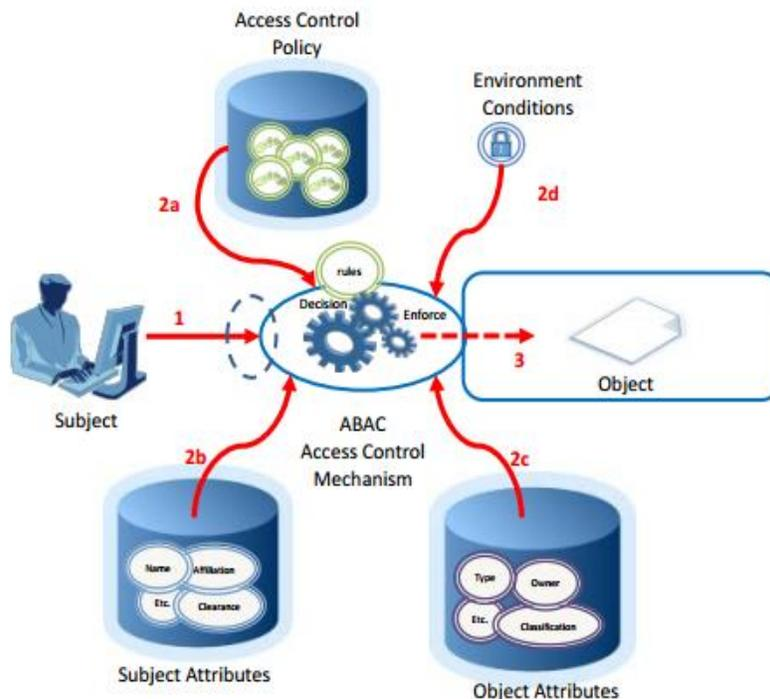
Figure 8: ABAC Basic Mechanism [16]
