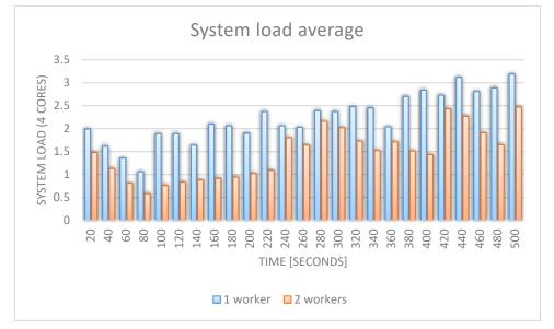
Figure 27. System load average of SensorData processing
