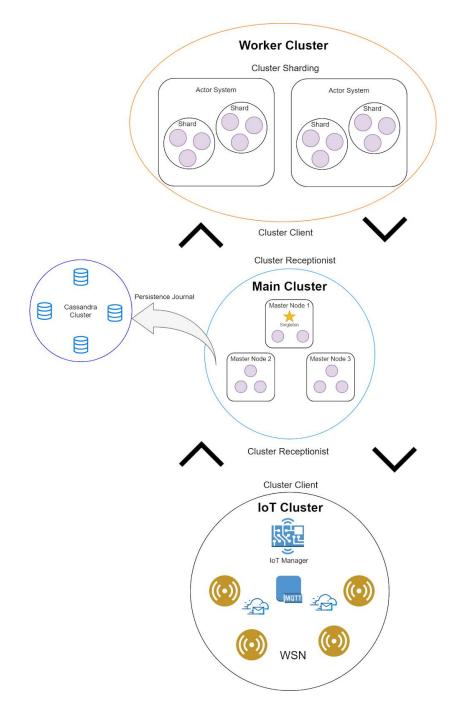
Figure 17. Akka IoT system architecture
