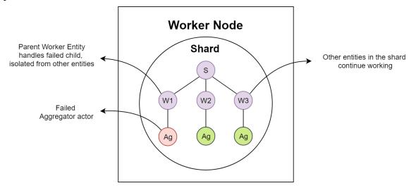
Figure 29. Isolation of failures on a shard
