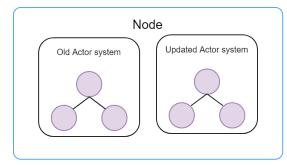
Figure 31. Two different actor systems deployed on the same node
