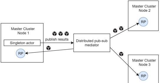
Figure 25. Distribution of results using Distributed pub-sub mechanism
