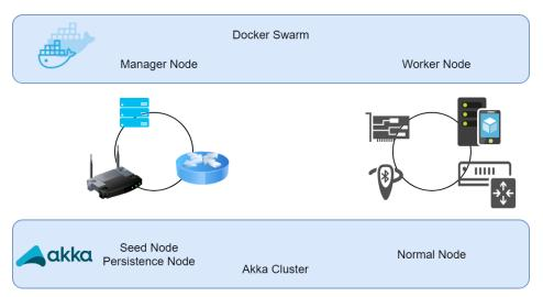
Figure 12. Mapping of Docker Swarm nodes to Akka Cluster nodes
