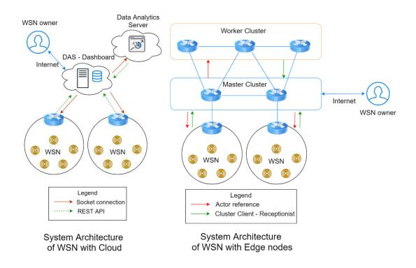
Figure 16. Cloud and edge IoT architectures
