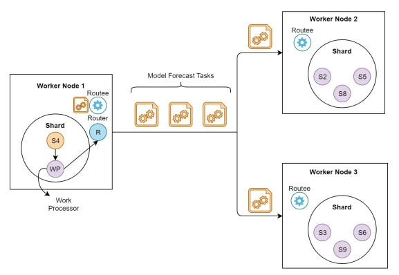
Figure 24. Distribution of computation tasks of a sensor entity in the Worker cluster
