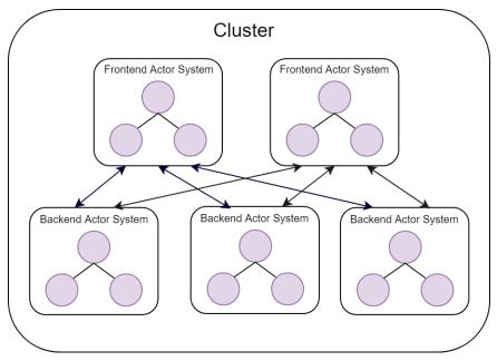
Figure 13. Cluster using Frontend and Backend actors
