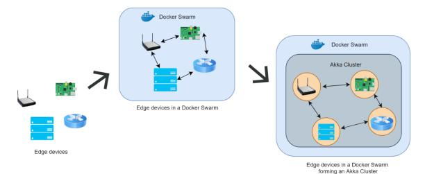
Figure 15. Edge devices forming an Akka Cluster in a Docker Swarm
