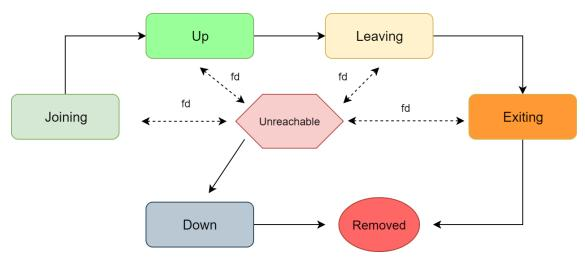
Figure 7. States of a node in an Akka Cluster
