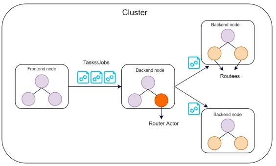
Figure 14. Cluster-aware routing with remote deployed routees
