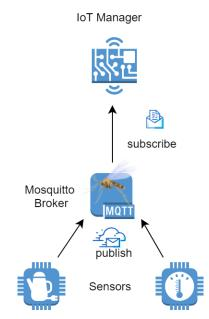
Figure 18. Publish-subscribe with MQTT broker on the IoT Cluster
