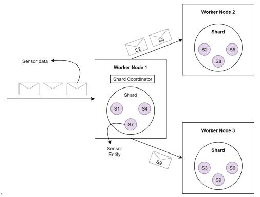
Figure 23. Distribution of sensor data in the Worker Cluster
