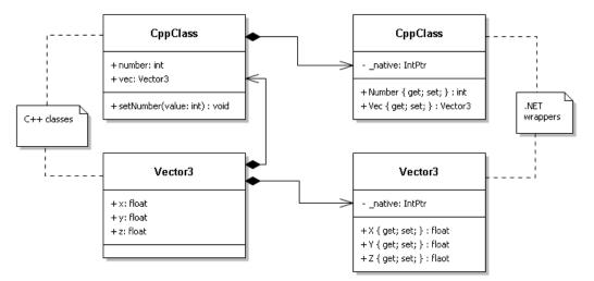
Figure 6: Wrapping C++ fields using .NET properties.
