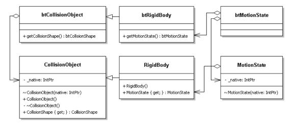
Figure 2 shows a typical class layout for unmanaged classes and their respective managed wrapper classes. *btCollisionObject* is an unmanaged class and *btRigidBody* is an unmanaged class derived from *btCollisionObject*. The managed wrapper class *CollisionObject* contains a pointer to the unmanaged *btCollisionObject* instance, which could also be a *btRigidBody* instance.
