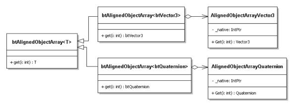
.NET generics do not support non-type parameters (e.g. numbers) either, so a C++ template specialization such as *btVector*<3> must be wrapped by a concrete class like *Vector*3.
